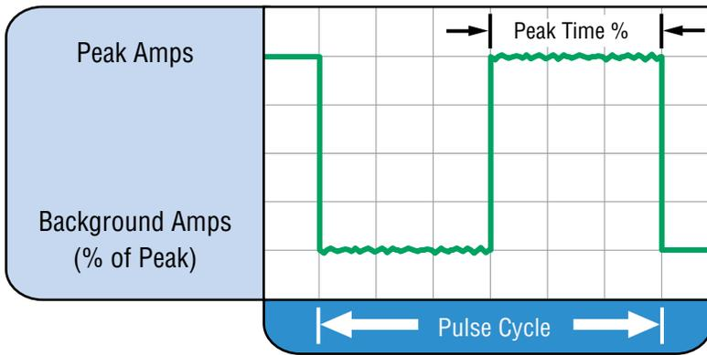
Typically from 1 to 10 pps. Provides a heating and cooling effect on the weld puddle and can reduce distortion by lowering the average amperage. This heating and cooling effect also produces a distinct ripple pattern in the weld bead. The relationship between pulse frequency and travel speed determines the distance between the ripples. Slow pulsing can also be coordinated with filler metal addition and can increase overall control of the weld puddle.
